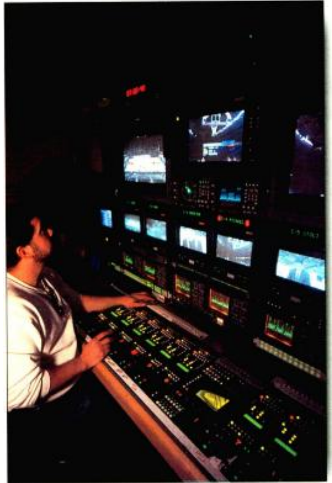
Camera control on HDV-5 is prewired for 12 cameras, including four Sony HDC-700 studio cameras and four HDC-750 portables, with additional cameras rented when required. Photo courtesy WRAL-TV.
