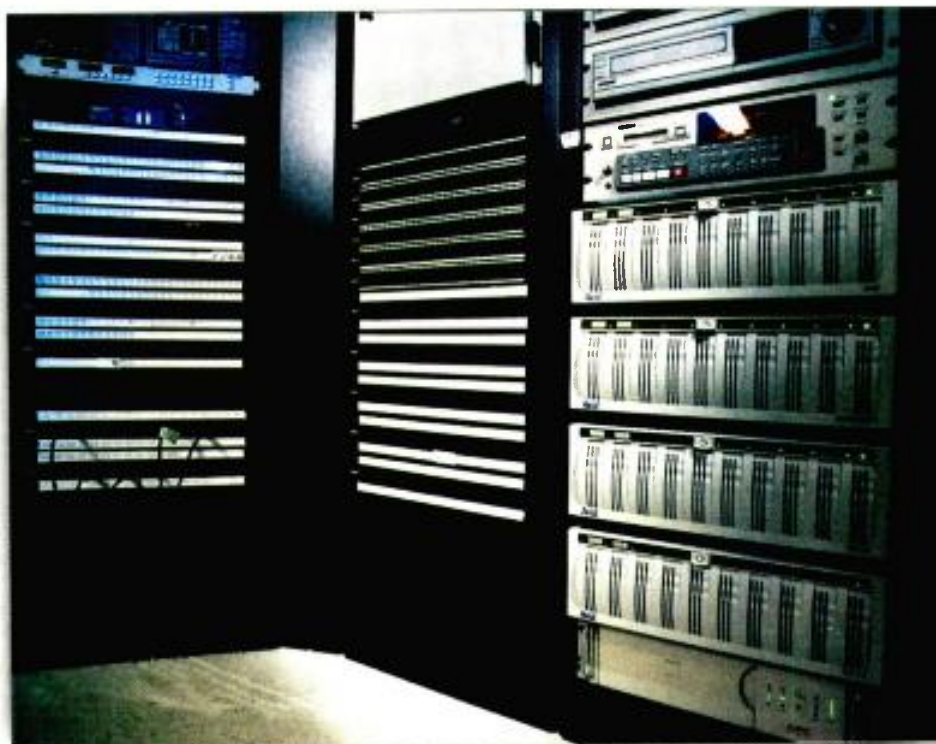
180Gb of shared fiber channel storage in the central machine room. Photo courtesy of Odyssey Network.
