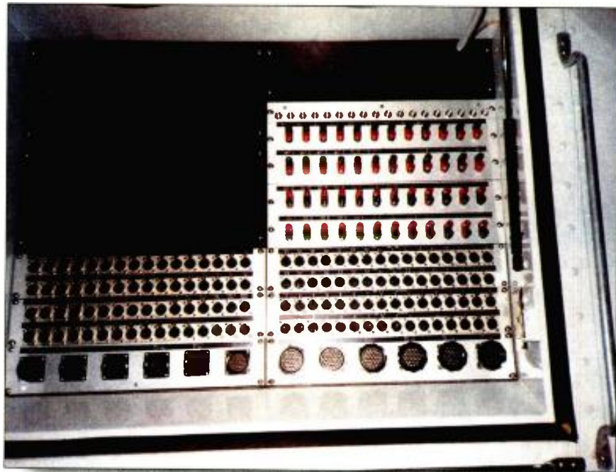
The majority of internal connections are available through patch panels for convenience and maximum flexibility.
